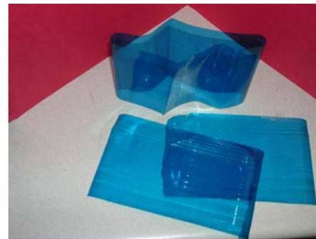
Plastic belts: dictation, monitoring (1940’s-60’s), folds, cracks, wear
