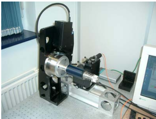
Figure 12: Top image is a schematic view of the scanning apparatus.. Lower left image shows overall setup including linear and rotational stages. In lower right image, confocal probe enters diagonally from the center right. Cylinder enters diagonally from the bottom center.
